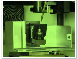
✤ The software is having a capability to set optimized laser power automatically according to the diamond size as well as for each individual process (Table cutting, Crown, Girdle and Pavilion).
